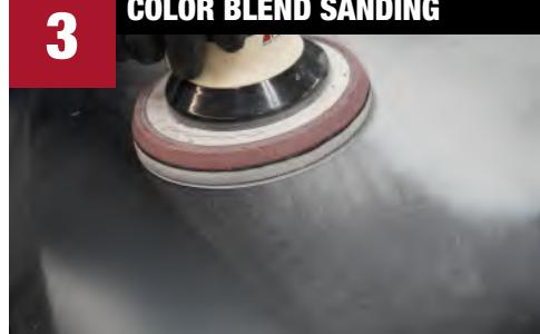
Sand color blend area with 800-grit sandpaper on a DA sander with a soft interface pad attached.
